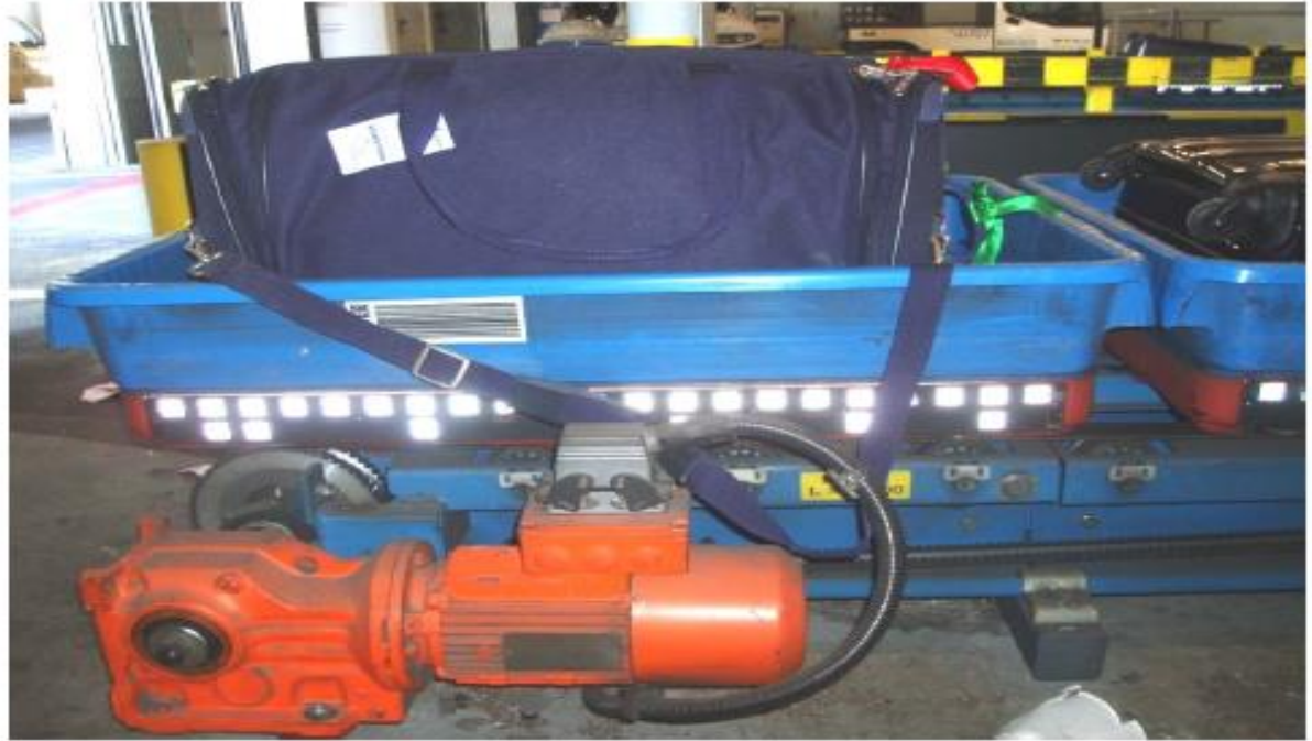
Straps entangled in a motor in the baggage handling system
