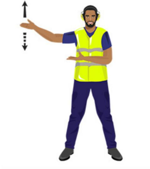
Stretch both arms toward load or equipment, palms up; hand movement in upward direction.
