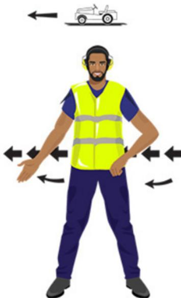
Come with load or equipment. Maintain eye-to-eye contact with operator/driver. Swing down opposite arm.
