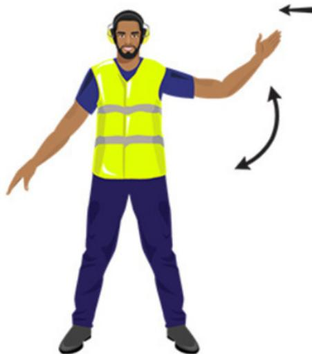
Right arm pointed downward, hand extended; left arm repeatedly moved upwards towards and downwards towards the guide person's right. Speed of arm movement indicates rate of turn.
