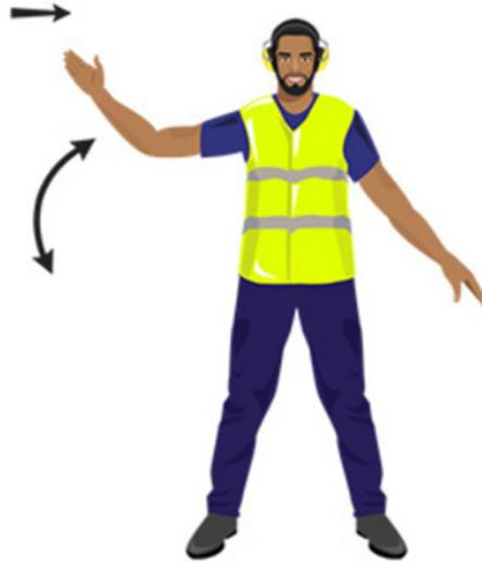
Left arm pointed downward, hand extended; right arm repeatedly moved upwards and downwards towards the guide person's left. Speed of arm movement indicates rate of turn.
