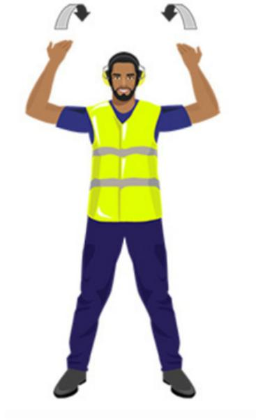
Arms held above the head with elbows a little bent and palms facing backwards; repeatedly move arms upwards and backwards, beckoning onwards.
