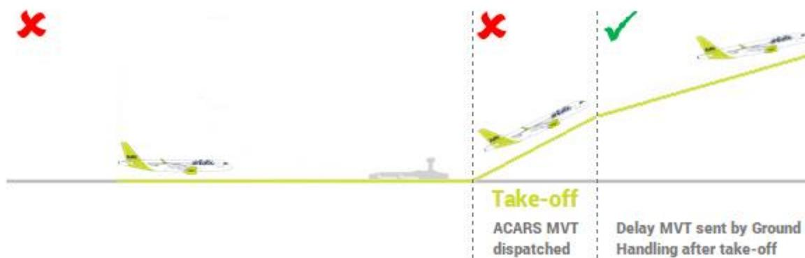
An automatic MVT is dispatched via ACARS during take-off. In case of delayed departure, delay code 99 (MX) is used. A copy of this MVT is also sent to Ground Handling partners. For Ground Handling partners it is necessary to send MVT for delayed flights only. Once MVT with applicable delay code received, existing MX in the system will be changed accordingly.
