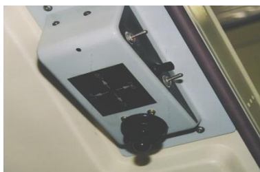
Joystick assembly inside the cargo hold door (ULD-holds)
