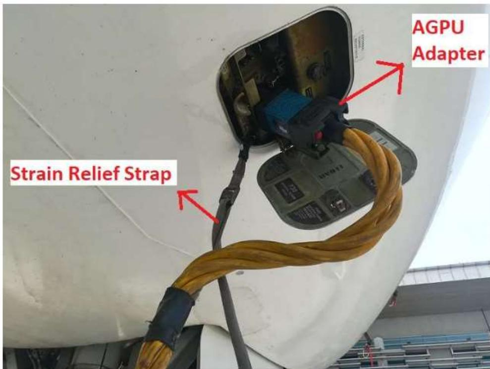
*Strain Relief Strap keeps the AGPU adapter from falling on the ground by its own weight. It hooks the AGPU cable with aircraft body.*
