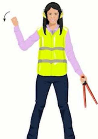
Raise hand just above shoulder height with open palm and, ensuring eye contact with the tractor driver, close into a fist. At the end of the pushback, also indicates to tug driver that aircraft brakes have been set. The tractor driver should return the signal to the headset operator to confirm vehicle brakes set.
