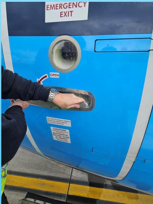
2. Continue turning to the direction of the arrow, the door will open outward
