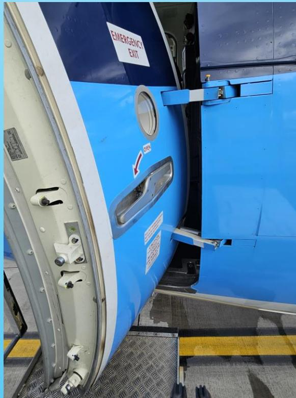
5. The handle will be flush reseated in its horizontal position
