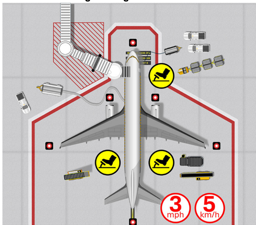
Figure 3.4 Precautions for Driving/Parking GSEs in ERA
