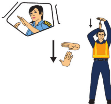
Figure 4-83: To disconnect power
