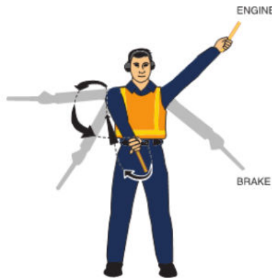
Figure 4-73: Fire - Communication During Engine Fire
