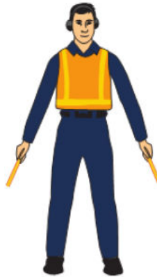
Figure 4-103: Hold movement of Aircraft
