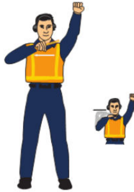
Figure 4-79: Emergency Engine Shut Down
