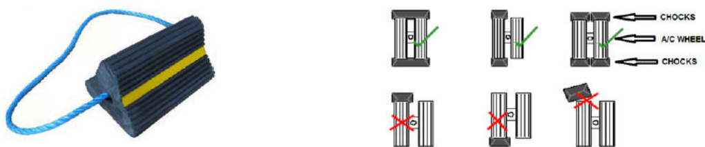
Figure 4-46: Parking Aircraft Out of Service/Night-Stop/High Winds
