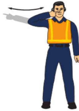
Figure 4-100: Change Of Pushback Direction
