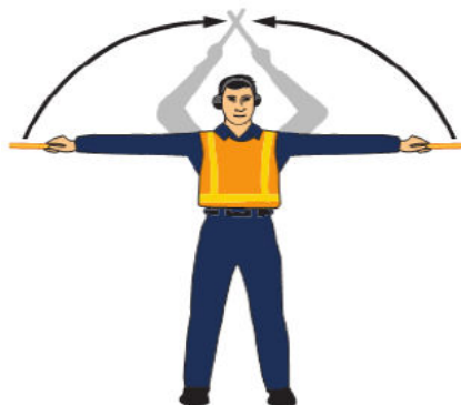
Figure 4-102: Stop movement of Aircraft
