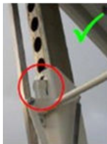
Figure 4-26: Pawl lock is correctly engaged.
