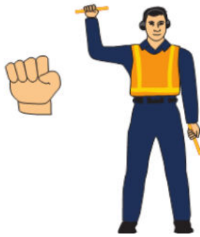
Figure 4-87: Do Not Touch Controls
