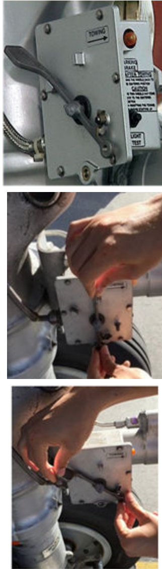
Figure 4-138: Figures of Electrical Box, Lever and Locking Pin
