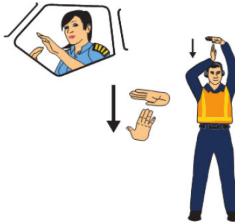
Figure 4-83: To disconnect power
