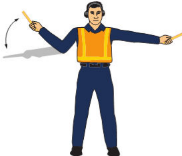
Figure 4-67: Turn right (from the pilots point of view)
