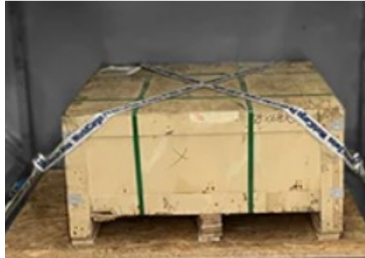
Figure 6-1: Load spreading on wooden board
