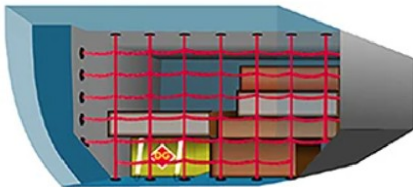
Figure 7-40: Example 3.c—Securing dangerous goods in a partially empty net sector
