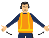
Arms down, hands closed facing outward, thumbs extended, move arms outward.
