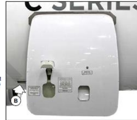
3 Press OPEN button on cargo door control panel to open door.
