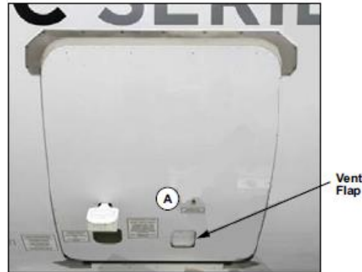
2 Push external handle up ensure vent flap opens and visual indicator shows red.
