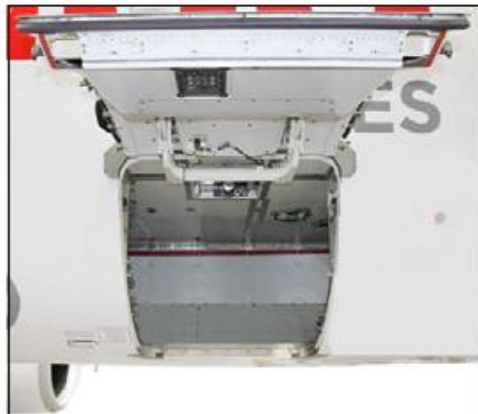
4 Door automatically stops when fully open.
