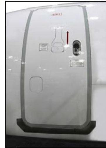
4 Ensure vent panel is closed and external handle is flush with the door.
