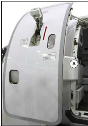
1 Pull the hold open handle to disengage the door.
