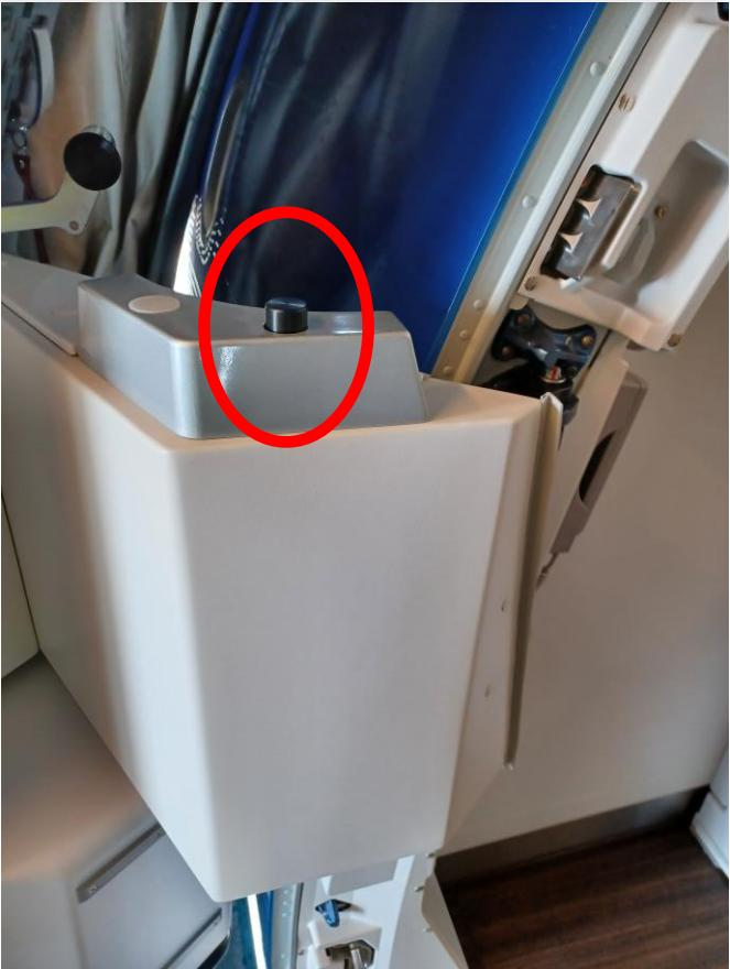
Before closing Door check that the platform is free of debris
