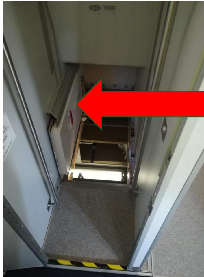
If the panel is in closed position, turn the red handle and block it as shown in the picture
