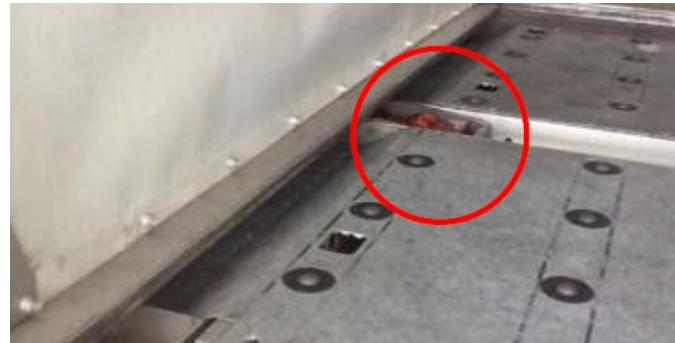
**A ULD is only secure when every required lock is fully engaged, serviceable, and verified.**
