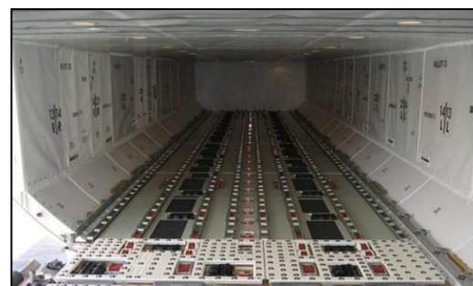
During the cargo compartment visual check, attention and care must be paid in order to avoid any possible damage. Report immediately any kind of damage or non-standard situations regarding the blow-out panels.
