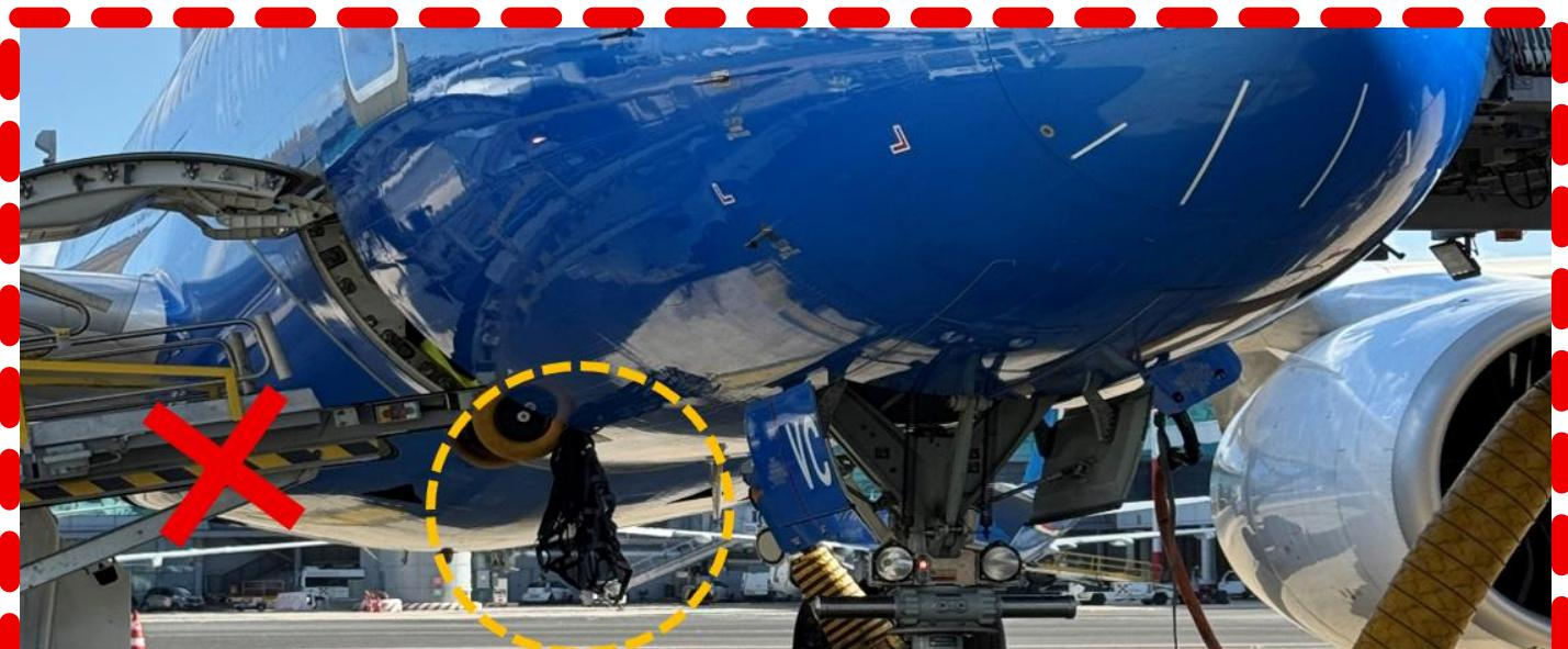
During handling, nets must **always** remain inside the compartment and must never hang outside, to prevent them from getting caught on equipment, being torn off, or picking up FOD that could damage the compartment.
