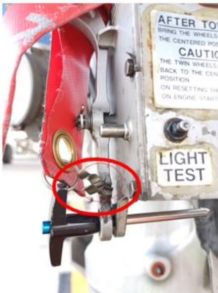
The photo clearly shows that this support is completely torn apart and detached from the towing box.
