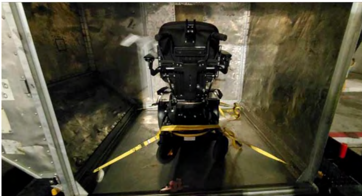
Figure 10. Power chair strapped by the base, alone in the container
