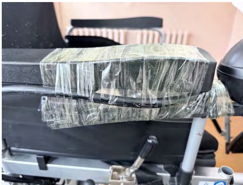
Figure 4. Example of Insulation of Wheelchair Battery Terminals
