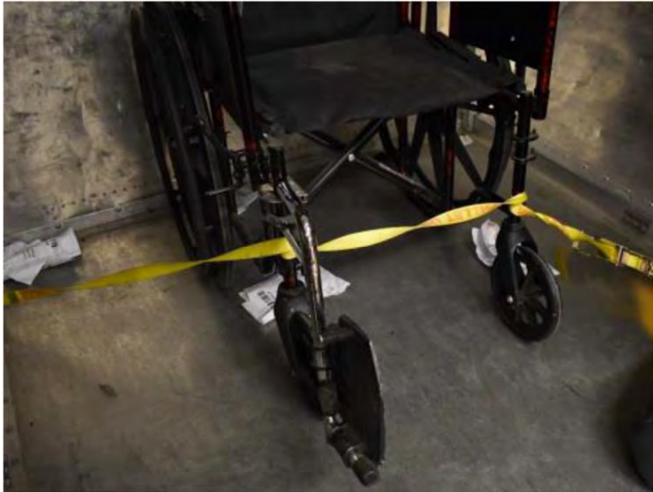
Figure 11. Securing the Mobility Aid Using Straps
