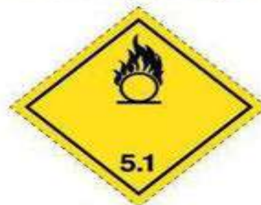
Name: Oxidizer Cargo IMP Code: RDX Minimum dimensions: 100 × 100 mm Symbol (flame over circle): Black Background: Yellow (Pantone Colour No. 109U) Figure 7.2.4 Class 5—Organic Peroxides (Division 5.2)
