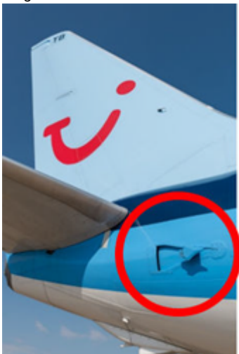
Boeing 737-800NG APU inlet door closed
