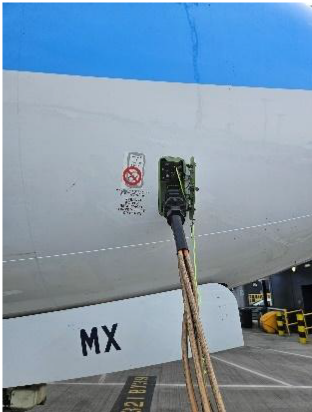
Right hand side service panel. NOTE; this is 2.5m above ground level.
