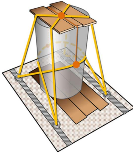
Figure 4.5.7.6.1. Lash barrels with protective planks
