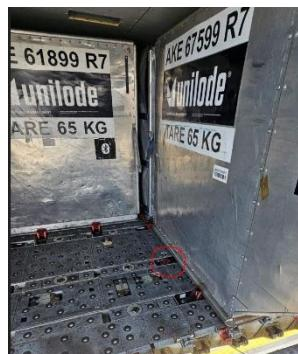
ULDs should be secured by a ULD restraint system on the compartment floor. Refer to the operator's GOM for relevant information on applicable ULD configurations, loading and restraint systems for each aircraft type.
