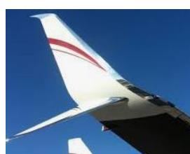
Please observe that B737-800 operated by JetTime with scimitar winglets and has additional requirements for placement of 3 safety cones. In front of, behind and outside the wingtip
