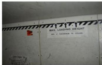
Ensure the necessary clearance between the load and aircraft hold ceiling is achieved to avoid any obstruction or damage to aircraft smoke detector/fire suppression system. Specific requirements given by the operating airline shall be followed.
