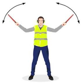
Wing walkers, if required, will be positioned approximately 1 m (3 ft.) outside the path of the wingtips. Wing walkers shall maintain visual contact with the marshaller until the aircraft has come to a complete stop.
