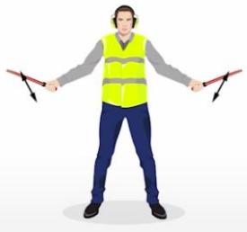
As the aircraft approaches the stop position, use the “Slow Down” signal, if required. As the nose wheel reaches the stop point, slowly cross the wands in the “STOP” signal.
