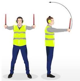
As the aircraft approaches the stand area, the marshaller points to the guide-in line on the ramp to be followed by the aircraft by standing at the top of the guide-in line and giving the “Identify Gate/Stand” signal.
