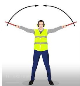
If at any time during the aircraft movement the marshaller is unsure or identifies an imminent danger, signal the aircraft to “STOP”.
