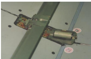
Continuous side rail, roller and tie down / net fixing point
