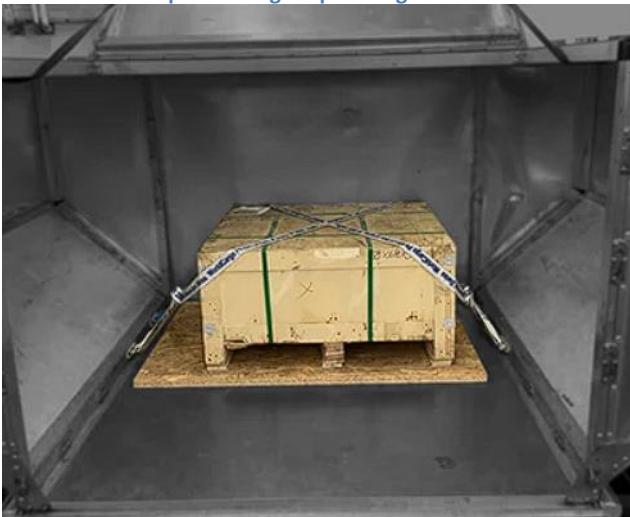
Picture 42. Example of Weight Spreading with Wooden Board
